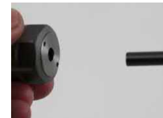
Insert cutting tool with the seal engaged on the round part of the shank
