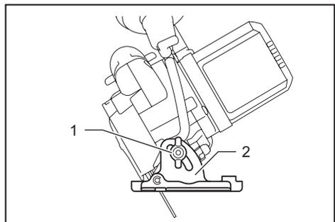
► 1. Clamping screw 2. Bevel scale plate
