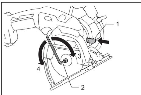
► 1. Shaft lock 2. Hex wrench 3. Tighten 4. Loosen
