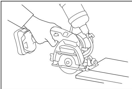
Hold the tool firmly. Set the base plate on the workpiece to be cut without the wheel making any contact.
