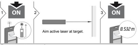
Target surfaces: Measuring errors can occur when measuring to colourless liquids, glass, styrofoam or semi-permeable surfaces or when aiming at high gloss surfaces. Against dark surfaces the measuring time increases.
