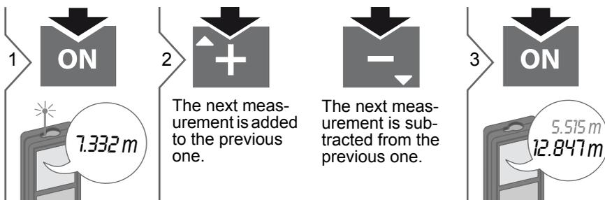
**i** The result is shown in the main line and the measured value above. This process can be repeated as required. The same process can be used for adding or subtracting areas or volumes.
