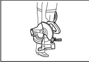
Carry the tool by carrying grip as shown in the figure. If you remove the holders, dust bag, etc., you can carry the tool more easily.
