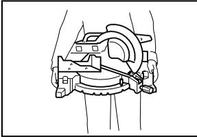
Carry the tool by holding both sides of the tool base as shown in the figure. If you remove the holders, dust bag, etc., you can carry the tool more easily.
