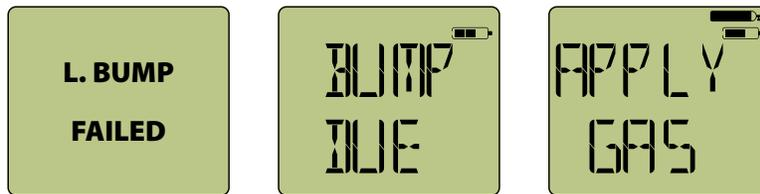
If a sensor fails the bump test, display will show "**Err**" and designate which sensor did not pass. The failed sensor will be disabled and will need to be replaced (see "**Err**" in **Failures/FAQ's** section).
