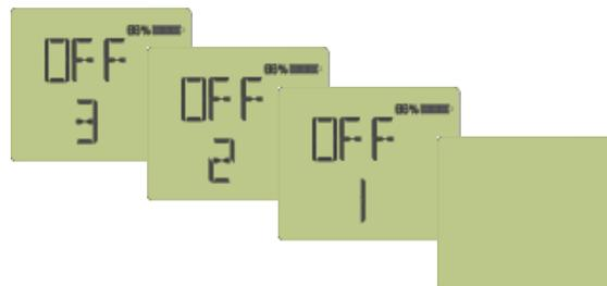
During the countdown, the detector will beep and flash 4 times. Release the button after the countdown and the detector will turn off.
