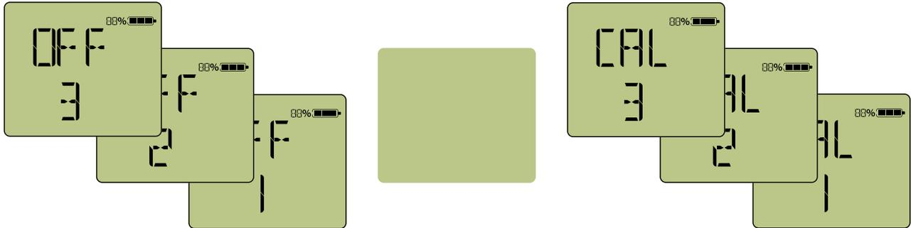
During these two countdowns, the detector will beep and flash 8 times with a pause between countdowns. Release the button after both countdowns are complete. The detector will first automatically zero the sensors at the current baseline reading, then the **"APPLY GAS"** prompt will appear. Display will show:
