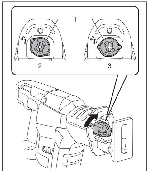
► 1. Blade clamp lever 2. Released position 3. Fixed position
