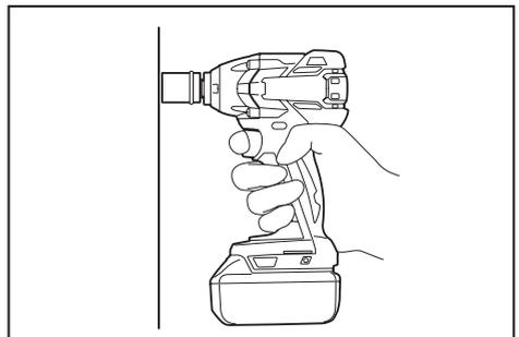
Hold the tool firmly and place the impact socket over the bolt or nut. Turn the tool on and fasten for the proper fastening time.
