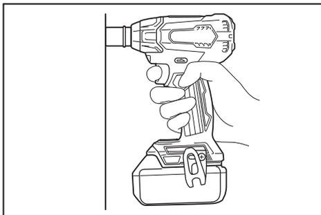
Hold the tool firmly and place the impact socket over the bolt or nut. Turn the tool on and fasten for the proper fastening time.
