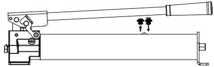
Remove shipping plug and replace with air vent plug (included) before initial use.
