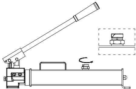
Turn the top cap counter-clockwise to open the vent before use.
